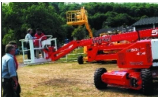
that of ours. The exceptionally high figure of 114 seconds for elevating speed is partially explained by the fact that this is a larger machine than the others and has about a metre more of boom. A final difference is that Snorkel describes the standard machine's slewing as being "continuous" – the particular model that we tested was being delivered the next day to a customer that had specified 358 degrees slewing.
